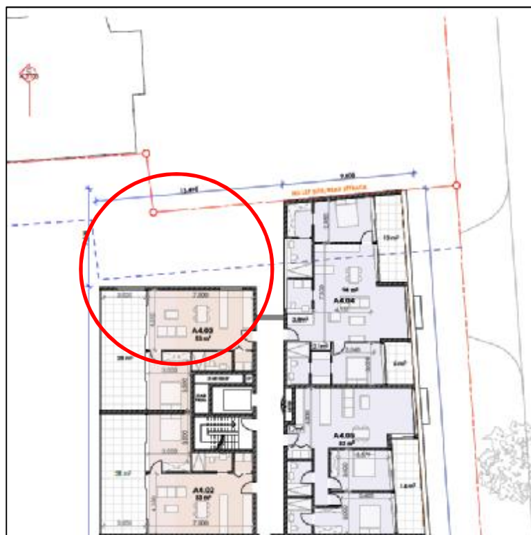
Figure 1 - Extract of Level 3 floor plan with red line indicating area of ADG setback (3F Visual privacy) variation which occurs over Levels 2-5 within Block A.
